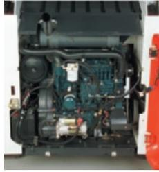
checks and fills, filters and battery. And unlike other brands, the lift arms need not be raised to service the machine. Shop time is spent repairing, not gaining access.
